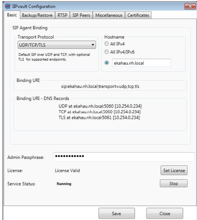
Figure 6: SIPvault Configuration, Basic Tab
