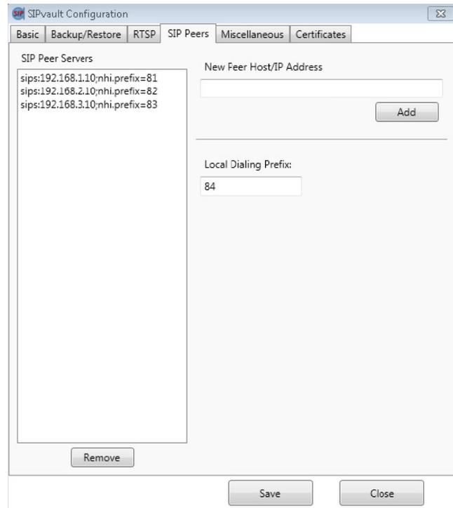
Figure 11: SIPvault Peer Configuration with Prefixes
